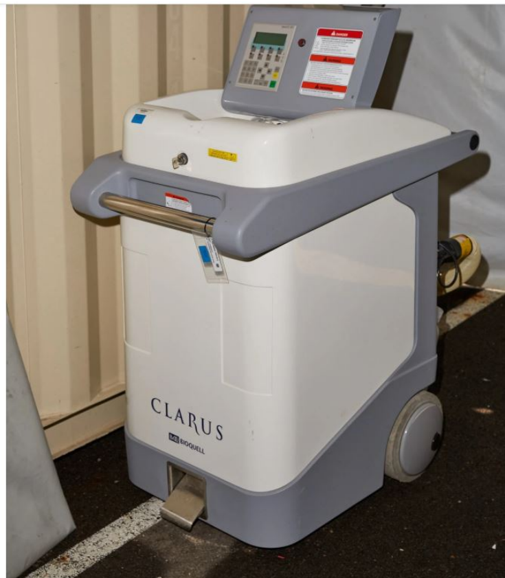
The hydrogen peroxide vapor decontamination unit used during the decontamination process.
