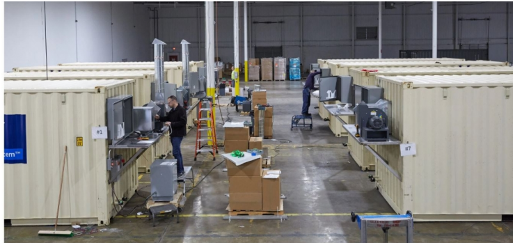
Battelle employees building decontamination chambers inside shipping containers.
