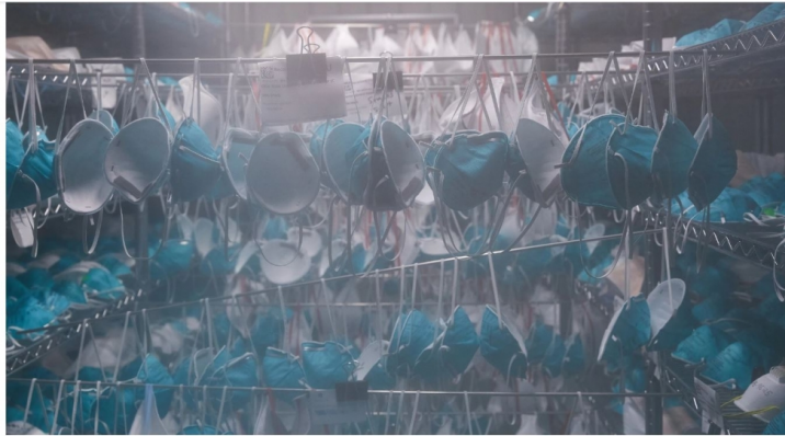
N95 masks and other protective equipment being decontaminated inside the chamber.
